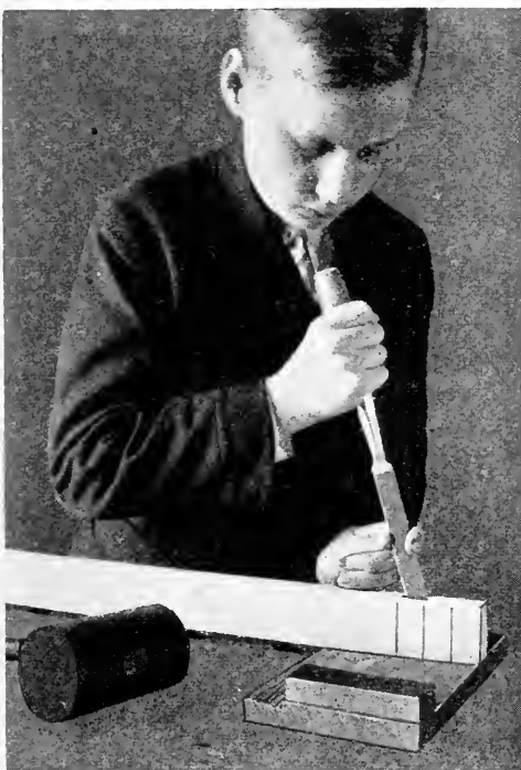
Fig. 20. Method for Holding Chisel in Mortising.
